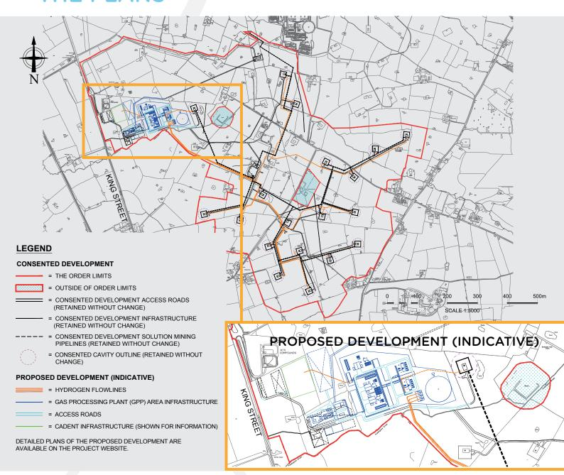
The KGSP would involve using specially designed underground salt cavities – created through solution mining – to store hydrogen.
